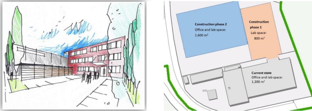
Figure 2: Architectural sketch of the laboratory building and site plan of the current laboratory and the two planned construction phases for the new building © ISC Konstanz e.V.
